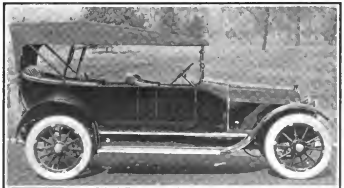
The Moon model 6-40 at $1,575 is now being built in six-passenger type, as illustrated. To accomplish this, the wheelbase has been lengthened to 122 inches, and the frame increased in size, and notwithstanding this, the weight of the six-passenger is identically the same as the five-passenger, namely, 2,950 pounds. Model 6-40 is equipped with a 3½ by 5 six-cylinder Continental motor, unit power plant, Delco starting and lighting system, etc.
